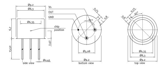
v-lambda weighted Si based VIS photodetector with integrated amplifier
