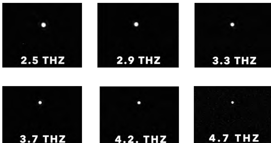
Fig 4. Measurement of focused beam for six different frequencies, after the auto-alignment module
