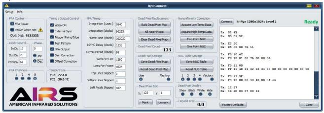
Enables a comprehensive set of tools for integrators, OEMs, and end users. This includes non-uniformity correction, dead pixel replacement, and four programmable NUC tables, in addition to the features included in Level 1 dashboard.
