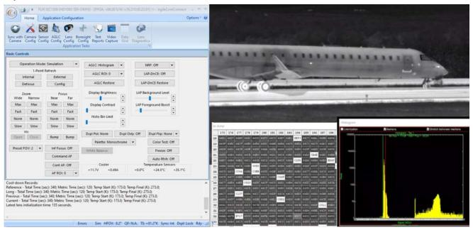
Provides a full suite of video processing options including lens control. A second video output channel can be configured to support HDSDI, GigE, HDMI, or USB3. Camera Link video is managed through a Imperx frame grabber, enabling live video management, scene ranges, pixel replacement and image enhancements.
