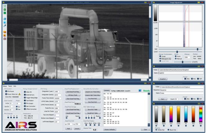
Offers comprehensive access and control over all system attributes and crucial image management, including proprietary AIRS contrast enhancement and pixel replacement tools. Advanced pixel correction features include intuitive tools that automatically identify and replace dead pixels, along with the capability to manually mark individual pixels. Select any of seven pseudo color palettes. Save snapshots or frame sequences in JPEG, PNG, or TIFF format.
