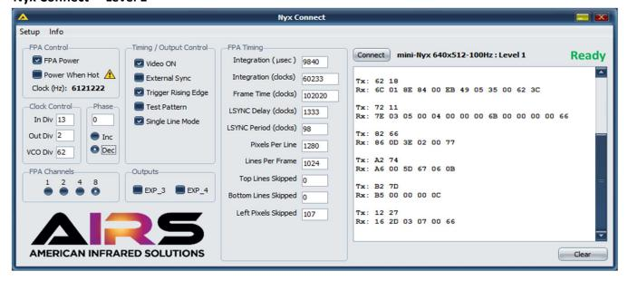
Ideally suited for Smart IDCA and Camera integration and enables streamlined development for engineers, systems integrators, and OEMs. The Nyx Connect software provides a user-friendly GUI enabling control over important camera and ROIC settings.
