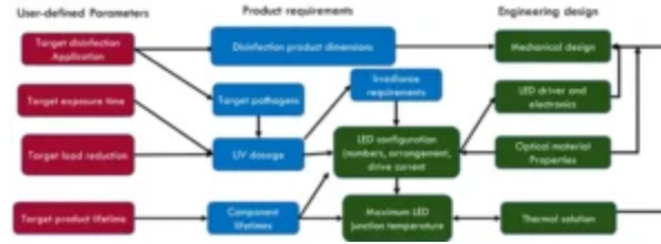
Figure 1: Device development process map showing interconnected design components.
