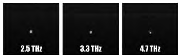
Figure 5 Measurement of the beam profile for three different frequencies, after the auto-alignment modules and a focusing lens
