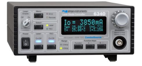
The 6300 Series ComboSource is a high-accuracy laser driver combined with a 60W temperature controller. With unique operational modes and safety features not found in other devices, this instrument is ideal for low and medium-power laser and LED applications.
