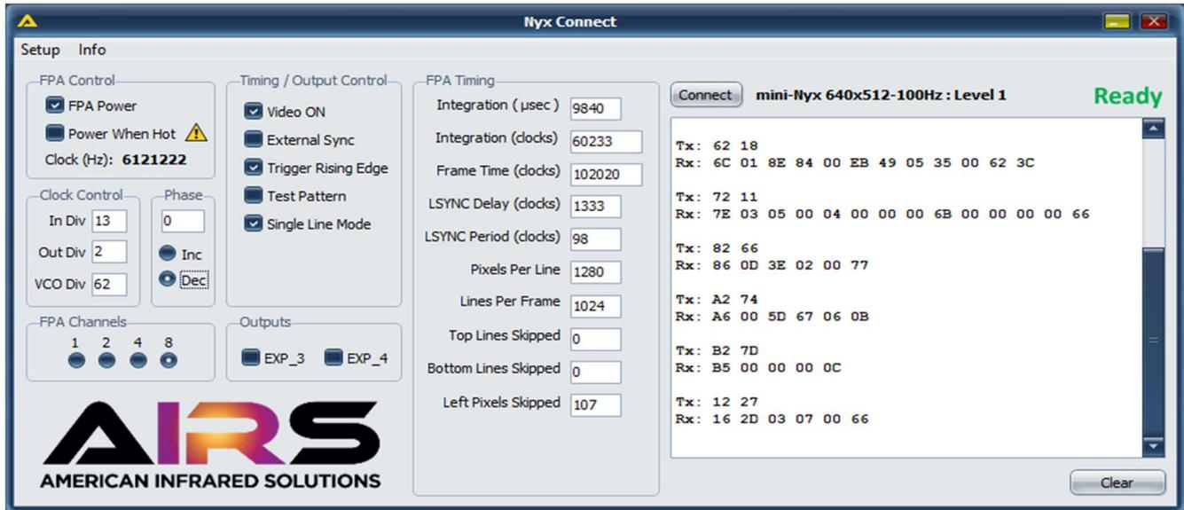
Ideally suited for Smart IDCA and Camera integration and enables streamlined development for engineers, systems integrators, and OEMs. The Nyx Connect software provides a user-friendly GUI enabling control over important camera and ROIC settings.
