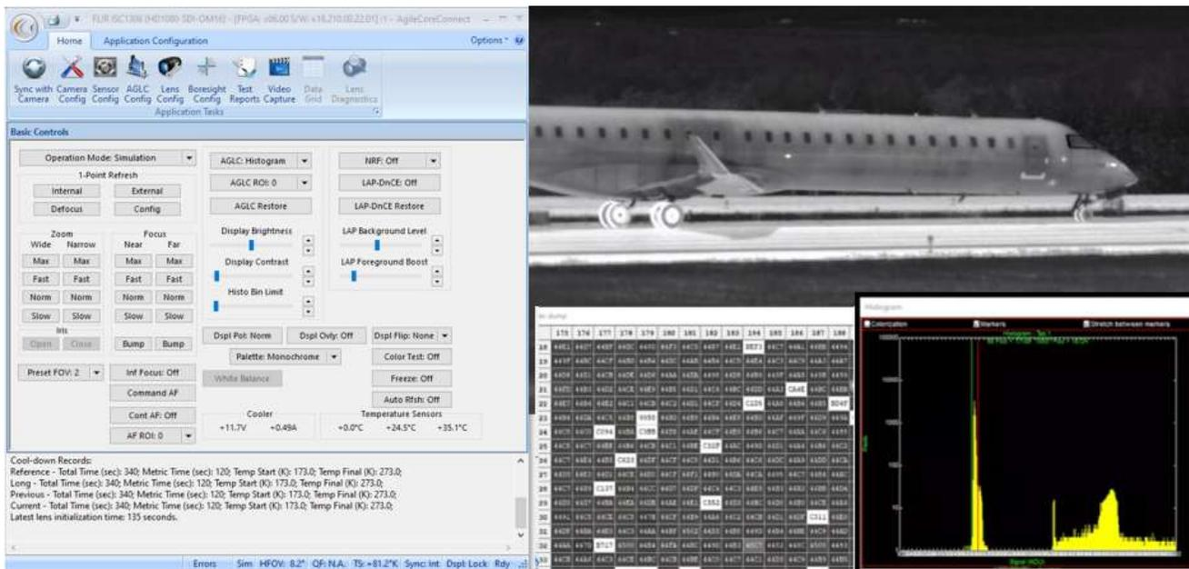
Provides a full suite of video processing options including lens control. A second video output channel can be configured to support HDSI, GigE, HDMI, or USB3. Camera Link video is managed through a Imperx frame grabber, enabling live video management, scene ranges, pixel replacement and image enhancements.
