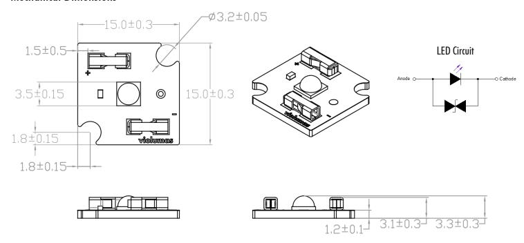
Note: The maximum offset (tolerance) for lens alignment over the LED is 0.2mm.
