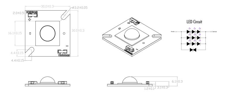
Note: The maximum offset (tolerance) for lens alignment over the LED is 0.2mm.
