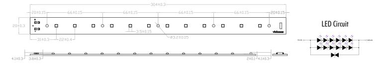
Note: The maximum offset (tolerance) for lens alignment over the LED is 0.2mm.
