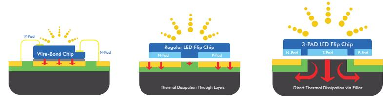
Violumas' groundbreaking technologies have the potential to transform the performance of the UV LED industry as thermal issues remain a persistent obstacle to achieving high optical power, particularly in the deep UV range, where up to 98% of energy can be dissipated as heat rather than optical radiation. Violumas is able to offer the most powerful UVC LED solutions on the market today with our expertise in thermal management and packaging solutions.
