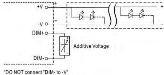
⊙ Applying additive 10V PWM signal (frequency range 100Hz ~ 3KHz):
