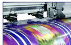
**Printing/Curing** UV LEDs save costs in curing with higher efficiencies, less electrical consumption, less heat, faster print cycles, and longer lifetimes compared to traditional lamps, and can be easily retrofitted into existing systems. UV LEDs also allow for design innovations in additive manufacturing systems, producing reliable parts with surface finish and mechanical properties. *Wavelengths: 405nm-365nm, 265nm.*
