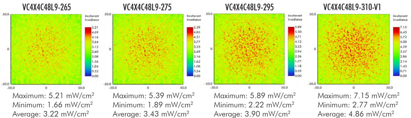
Irradiance plots below are simulated at throw distance of 10 mm and detector area of 100 cm<sup>2</sup>.
