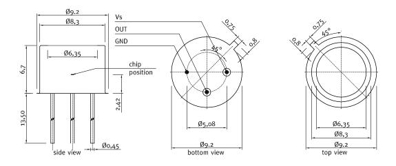
Broadband SiC based UV photodetector with integrated amplifier
