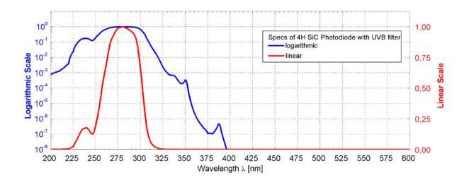
UVB+UVC SiC based UV photodiode A = 1.0 mm<sup>2</sup>
