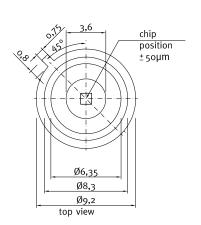
UVB+UVC SiC based UV photodiode A = 1.0 mm<sup>2</sup>
