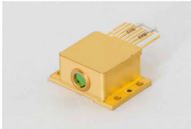
Picture of a HHL with collimated beam output. The lens is inside the housing, protected by a tilted window with AR coating.
