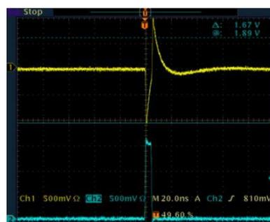
Response of A-PPI-D (yellow curve) to a positive pulse (cyan curve). Left short input pulse with 1 ns pulse width and right long input pulse with 5 ns width.
