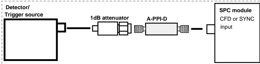
**Fig. 3:** If the trigger source does not work without a ground return path through the connected parts, a 1dB attenuator can be inserted. Such an attenuator with SMA connectors is available from bh.
