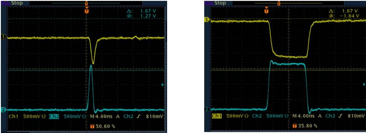
**Fig. 4:** Response of A-PPI to input signals with different pulse width. Left: 1 ns pulse width; right: 10 ns pulse width.
