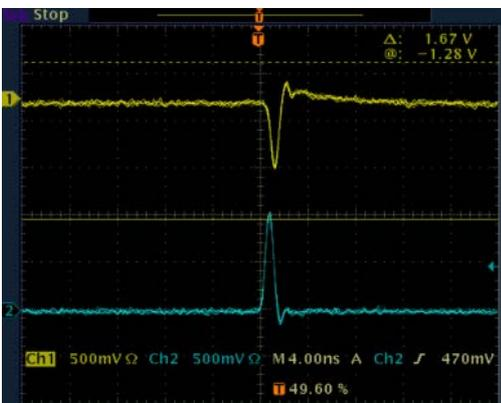
**Fig. 1:** Response of A-PPI-D to a positive pulse with a width of 1 ns. The output is a single negative pulse. Yellow: A-PPI-D output signal. Blue: input signal to A-PPI-D.
