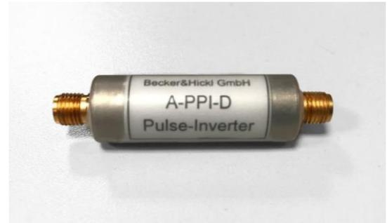
The A-PPI-D is a passive device used to transform positive pulsed signals such as TTL output pulses of detectors or trigger sources into signal pulses suitable for accurate detection with bh TCSPC modules.
