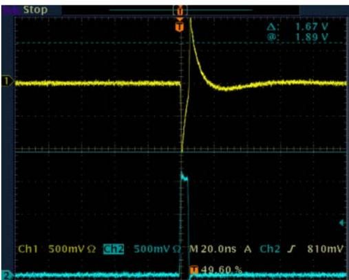
**Fig. 2:** Yellow: Response of A-PPI-D to a rectangular pulse with a width of 5 ns. Blue: Input signal, 5 ns rectangular pulse. The rising edge of the input results in a negative output pulse; the falling edge results in a positive pulse. In this case, the A-PPI-D delivers the derivative of the input signal. This way, the user can select the required polarity (normally negative).
