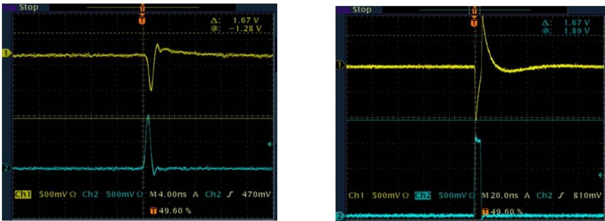
**Fig. 5:** Response of A-PPI-D to input signals with different pulse width. Left: 1 ns pulse width; right: 5 ns pulse width. In contrast to the A-PPI (Fig. 4) the A-PPI-D builds the derivative of the input for longer pulse widths which results in a double-peak structure.
