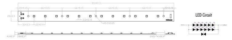
Note: The maximum offset (tolerance) for lens alignment over the LED is 0.2mm.
