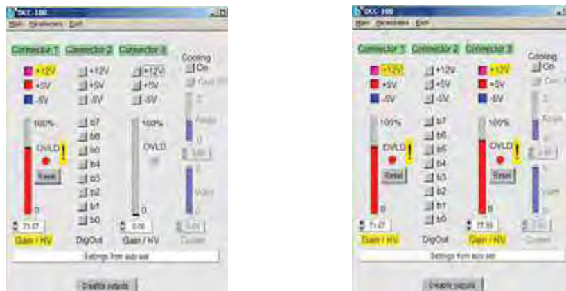
Fig. 11: DCC-100 panel after overload shutdown. Left one detector. Right: Two detectors, both detectors shut down.
