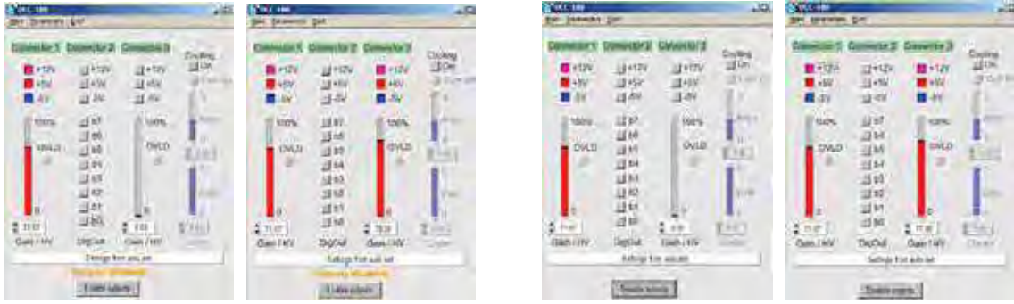
Fig. 9: DCC-100 control panel, for one detector and for two detectors. Left: After software start, the detectors are disabled. Right: Detectors enabled. The ‘Gain’ sliders control the AD voltages.
