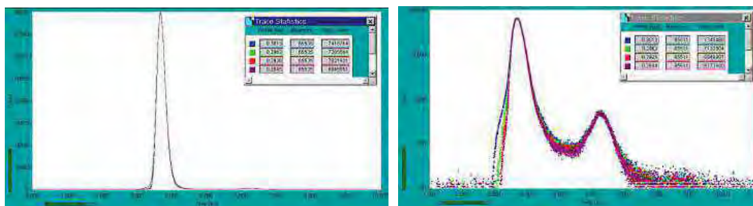
Fig. 23: H7422-40, TCSPC Instrument response function. Gain control voltage 0.9V (maximum gain), preamplifier 20dB, discriminator threshold -200mV, -300mV, -400mV and -500mV
