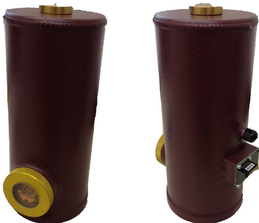
Figure C.1.: A LN2 dewar. The light output is seen on the left, the LBI connector on the right.
