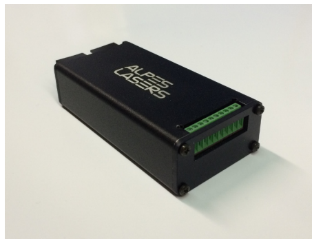
Figure 5.8.: S-2 pulser in eloxed aluminium box.
