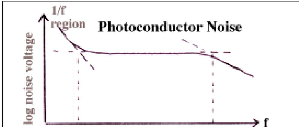
To predict low frequency performance of a photoconductor, the extent to which  $D^*$  is degraded by  $1/f$  noise must be estimated. Either of the following ways is applicable:
