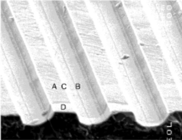
Fig. 7. SEM images of a multi-heterojunction photodetector: plan view of the whole device. A – mesa structure, B – trenches, C – non-metallised wall, D – non-metallised region of the device.
