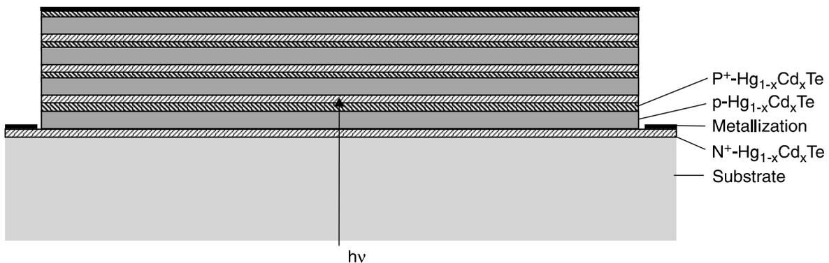
Fig. 8. Schematic cross-sections of single N<sup>+</sup>-p-P<sup>+</sup> heterojunction photodiode cell (a) and the 4-cells stacked multiple detector (b). The backside illuminated device is supplied with reflector for double pass of IR radiation.
