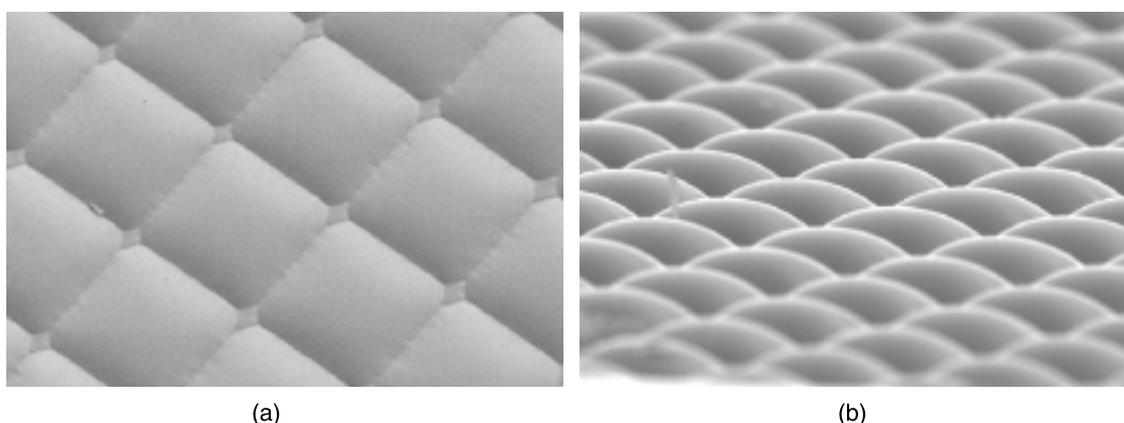
Fig. 4. SEM images of the microlens array: top (a) and tilted side view (b). The size of the individual lens is 50×50 μm.
