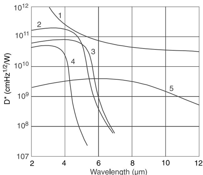
Fig. 9. Spectral detectivity of advanced photoconductors and photovoltaic devices: 1 – background limit  $D_{BLIP}^*(300 \text{ K}, 180^\circ)$ , 2 – PCI-2TE-5, 3 – PDI-2TE-5, 4 – PDI-4, 5 – PCI-2TE-10.6 (After Ref. 23). The symbols stand for: PC – photoconductive, PV – photovoltaic, I – optically immersed, 2TE – two-stage Peltier cooling.
