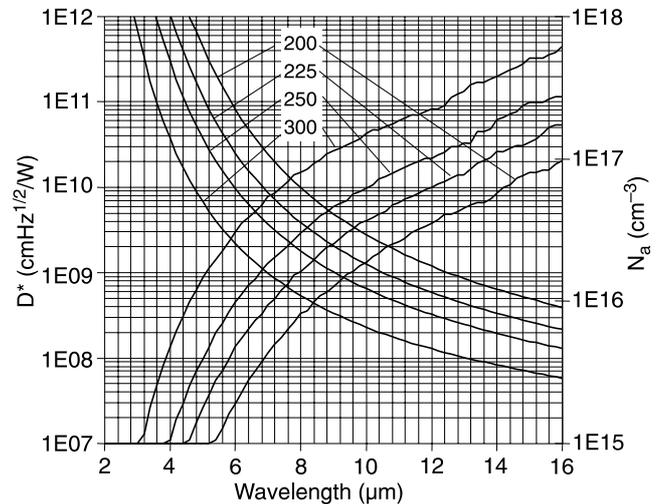
Fig. 3. Ultimate performance of  $\text{Hg}_{1-x}\text{Cd}_x\text{Te}$  photodetectors and optimum acceptor doping as a function of wavelength and temperature (double pass of radiation is assumed).
