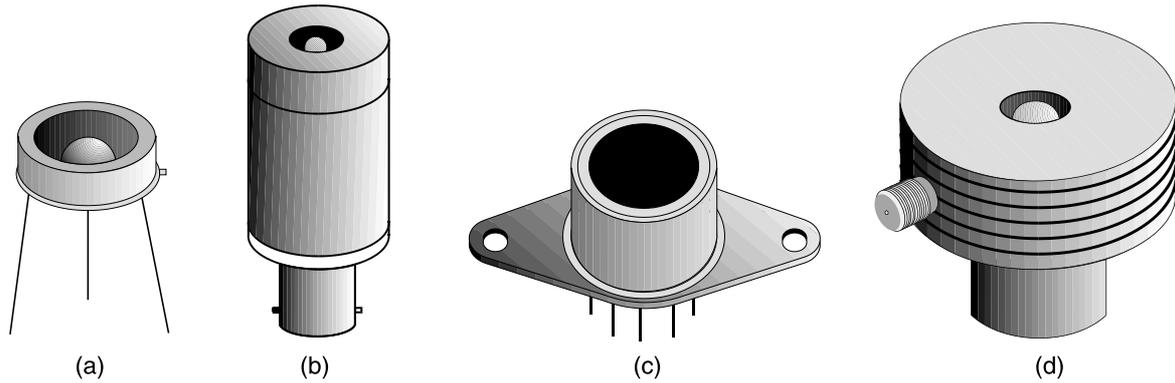
Fig. 5. Housings of optically immersed MWIR and LWIR  $\text{Hg}_{1-x}\text{Cd}_x\text{Te}$  photodetectors: uncooled optically immersed photoconductors and photodiodes  $f < 30$  MHz (a), uncooled optically immersed photoconductors and photodiodes  $f > 30$  MHz (b), Peltier cooled photoconductors, and photovoltaic detectors (c), photoelectromagnetic detectors (d) (after Ref. 22).
