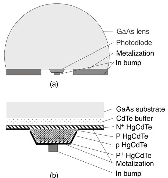
Fig. 6. Schematic cross-section of optically immersed  $10.6 \mu\text{m}$  mesa photodiode for operation at 200–300 K: complete structure (a) and enlarged view of active element (b).
