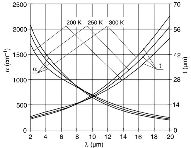
Fig. 2. The calculated absorption coefficient and thickness of optimised photodetectors as a function of operating wavelength and temperature (single pass of radiation).
